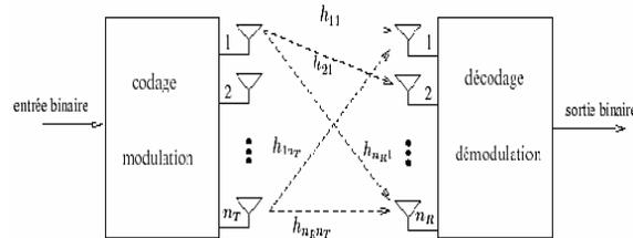
Fig (1) Principle of a MIMO system
