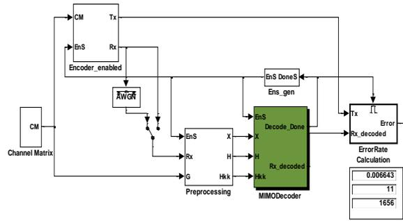
Fig (4) decoding algorithm using Simulink
