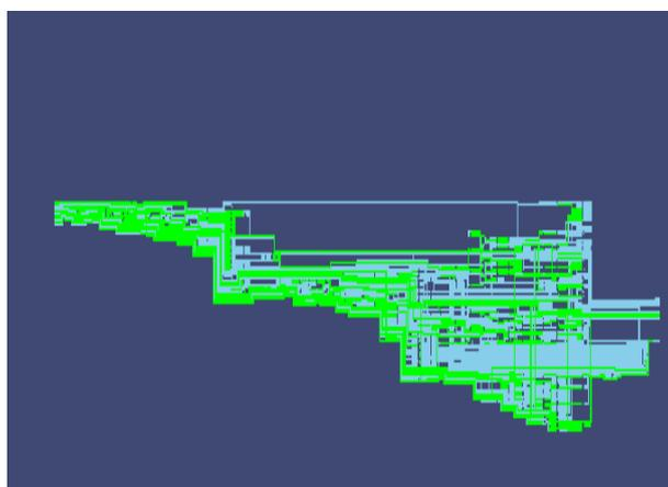
**Fig (9) MIMO decoder after placement / routing on Xilinx Virtex 4**
