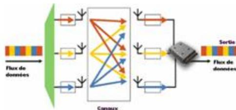
Fig (2) Principle of spatial multiplexing
