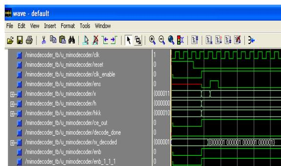
Fig (7) the timing associated with MIMO decoder
